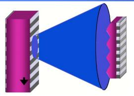
Polarizing nanostructures are 0.5% the thickness of the conventional polarizers used in current isolator manufacturing processes. Use of the thinner polarizing nanostructures enables isolators to be manufactured in smaller configurations, and dramatically lowering pricing.
